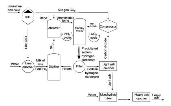
The Solvay process manufactures three different products - light sodium carbonate (light ash), granular sodium carbonate (heavy ash) and refined sodium hydrogencarbonate.
